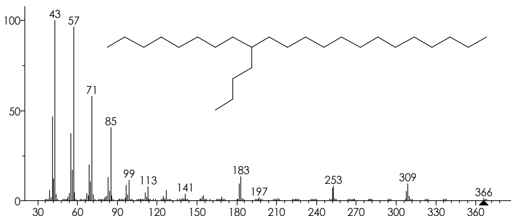
Figure 6-15. EI mass spectrum of 9-butyldocosane, a branched aliphatic hydrocarbon.
