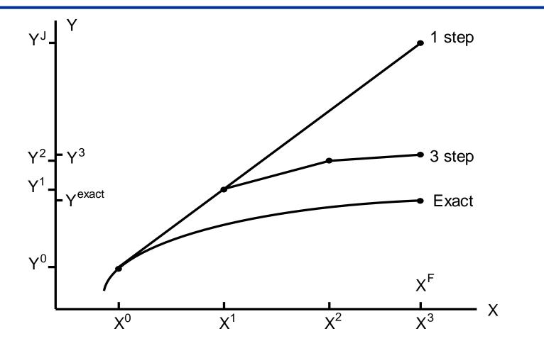
Multi-step process to reduce linearization error
