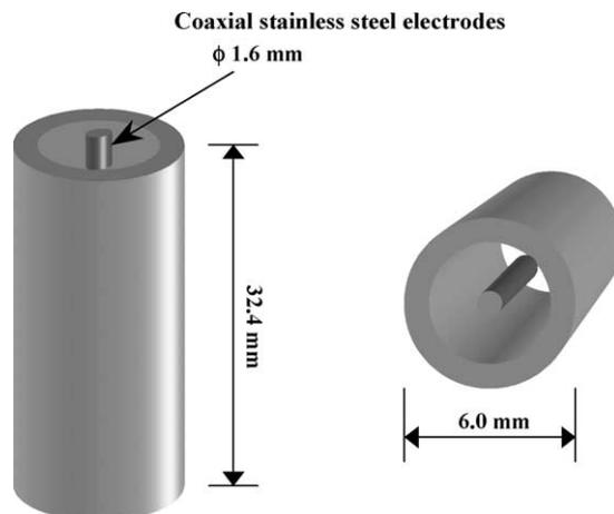
Fig. 1. Schematics of the impedance transducer.
